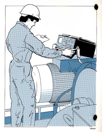
ols; Phase Analysis; Scan Analysis; Time Averaging; Exernal Sampling etc. allow the machine operator to make qualitative assessments of machine condition on-the-spot.
