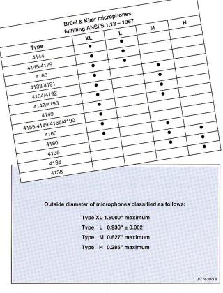
Other standards relevant to general-purpose microphones are those for sound level meters. This is because the sound level meter ratings (e.g. Type 0, Type 1 etc.) usefully reflect the accuracy and environmental robustness of the accompanying microphone. The table opposite lists the Brüel & Kjær microphones which fulfil the requirements of the sound level meter standards. The various sound level meter 'Types' are summarized below.
