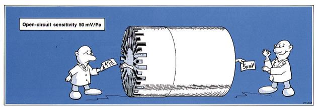
The chain of procedures used in the factory-calibration of opencircuit sensitivity together form a calibration 'hierarchy'. At the top of the Brüel&Kjær hierarchy are the **primary-standard** microphones — on whose accuracy and reliability all other links in the chain depend. The Brüel&Kjær 'primary standards' undergo absolute calibration once a year by an independent institution — the National Bureau of Standards, Washington DC.
